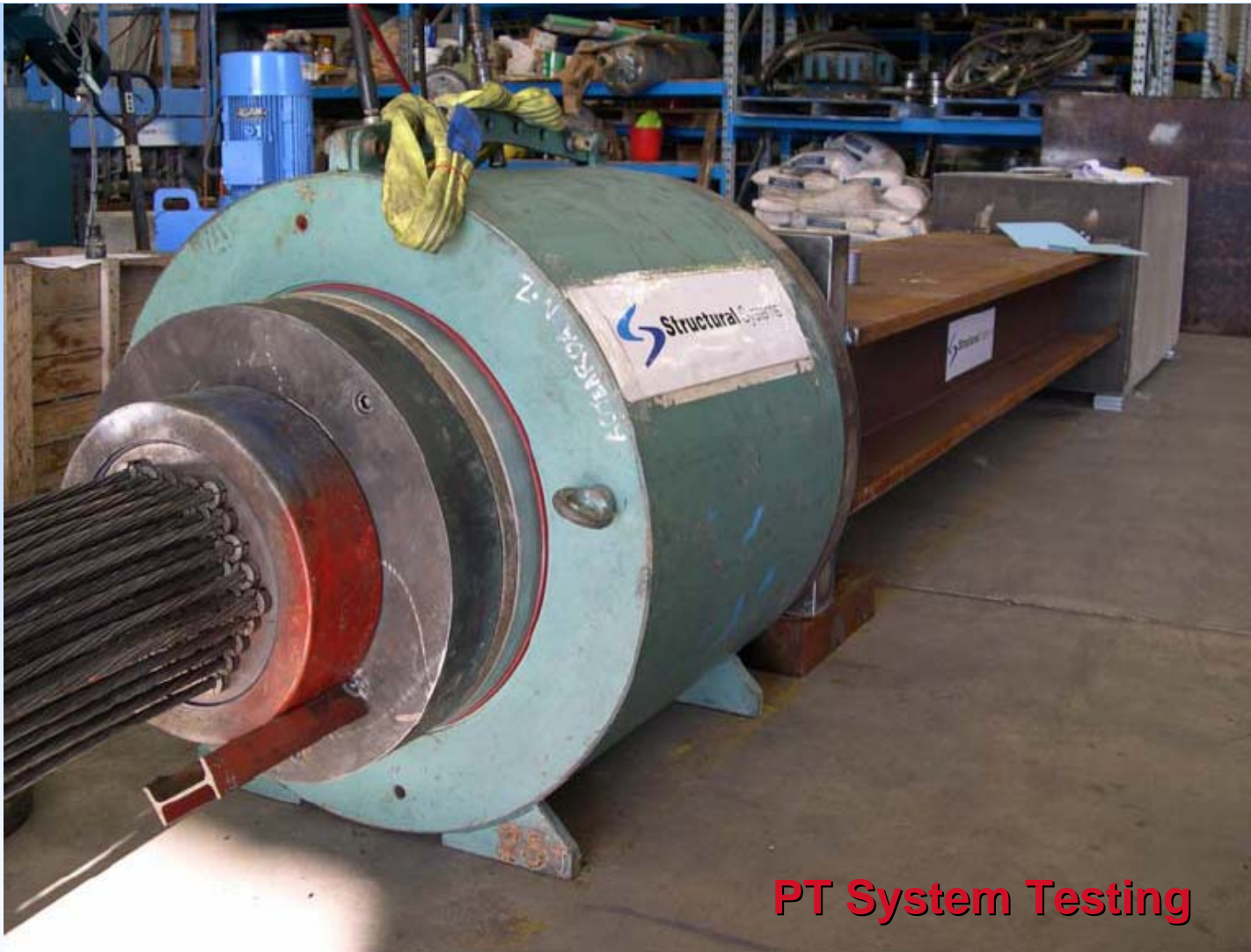
Photo D3: Anchor block test set-up viewed from the jack end Specimen 6105-01
